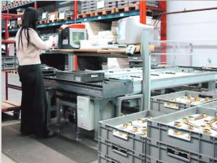
The polished fittings are stored in the automatic buffer warehouse on an ongoing basis
