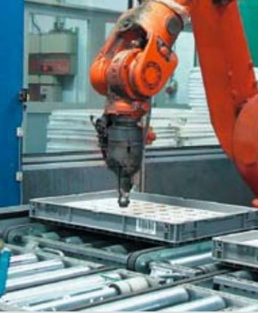
Left photo: The robot reaches into the container in order to treat the rough fittings, one after another, with sanding and polishing agents. The container content is 'recognized' by a camera and finished off one by one
