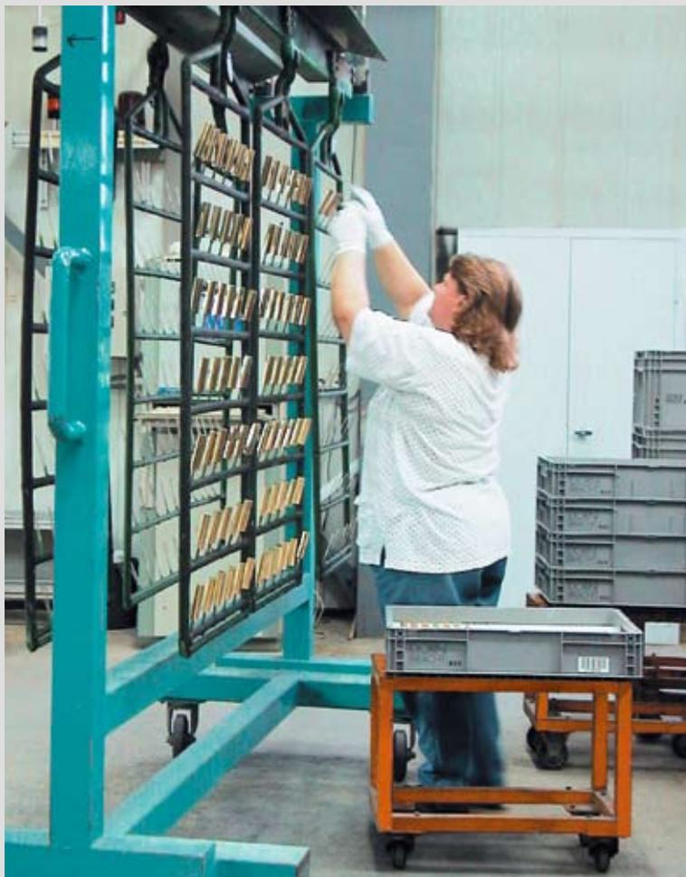
The polished goods are sent from the automatic warehouse to the electroplating area. For plating, the fittings are placed individually on a goods carrier or electroplating racks
