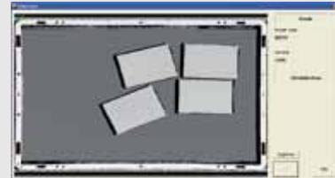
The image recognition system especially developed for the SRP determines the position of the products on the storage trays.
