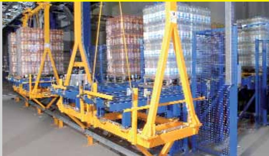
In the intermediate building the Euro pallets are taken off the monorail, the Düsseldorf pallets are separated and transferred back onto the monorail.
