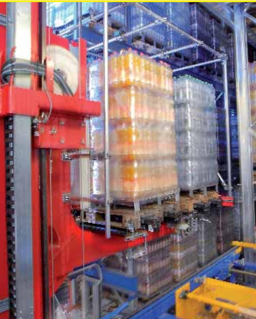
The SRMs can retrieve two Euro pallets loaded with two Düsseldorf pallets each and transfer them to the monorail.
