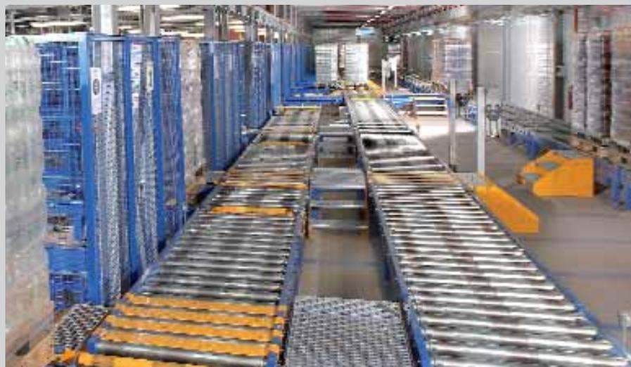
The integrated conveyor system forwards the pallet with beverages directly to the high bay warehouse for storing.
