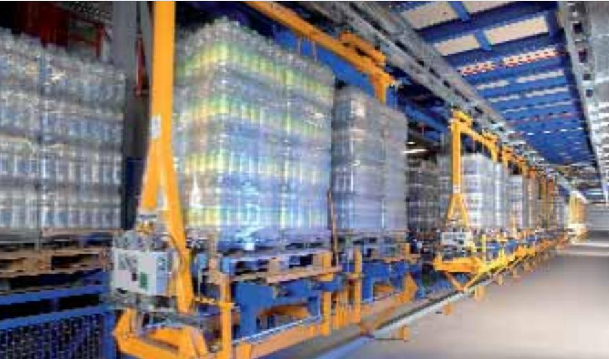
The trolley of the approximately 350 meter long electric monorail can transport two Euro pallets at a time.
