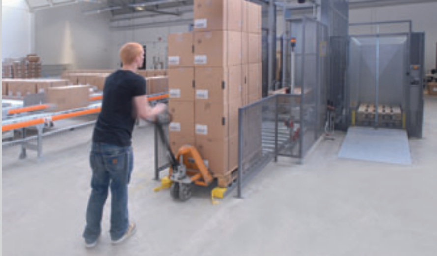
The packed pallets can be conveniently removed from the palletizer with forklifts.
