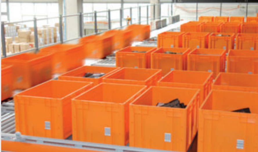
The bins are conveyed via a sorter to the order-picking locations and back to storage in AKL.
