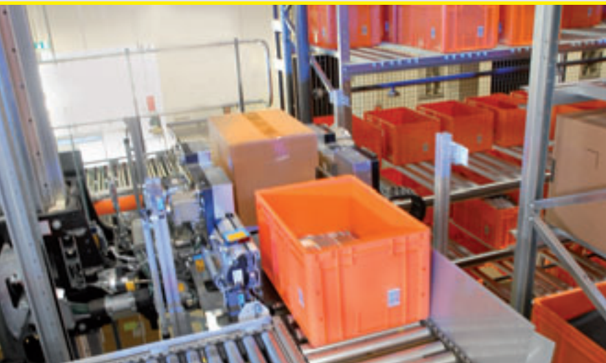
With a Twister V load-carrying devices the SRMs are able to store and retrieve two different load units double deep.
