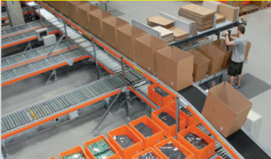
If necessary, several orders can be parallel picked at four order-picking locations.
