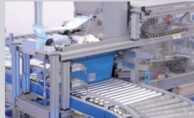
Exact and continuous weight checks with check stations ensure **quality control** of the picking processes at all picking areas. Separate check stations for picking cartons and totes before they continue to address insertion station and shipping once again ensure that the high requirements of GEHE to reach a zero-error target are met.
