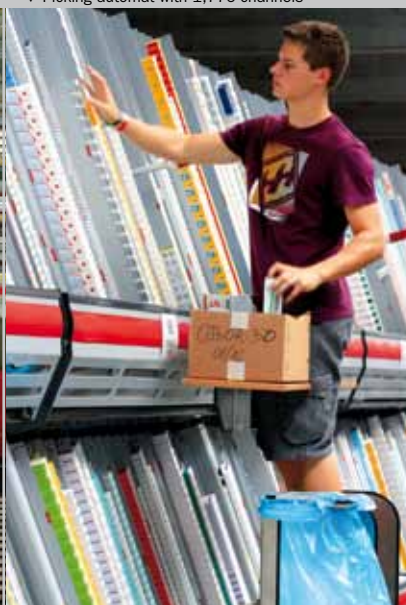
▲▼ Picking automat with 1,776 channels
