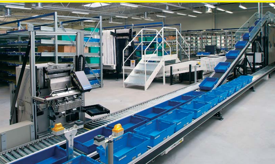
Conveying system with note insertion
