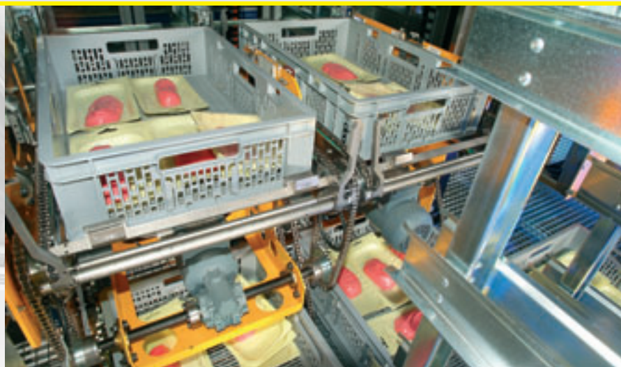
Transport of shipping bins by the load-carrying device of SQS with quadruple extracting device
