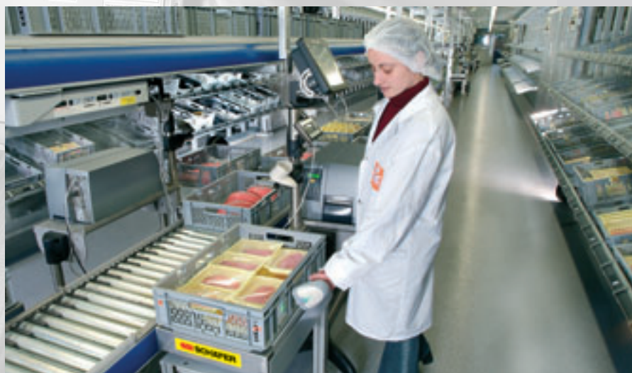
Pick by Light order picking in the finished goods warehouse
