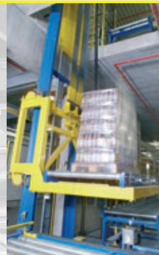
The pallets are transported between two levels by a total of four vertical conveyors
