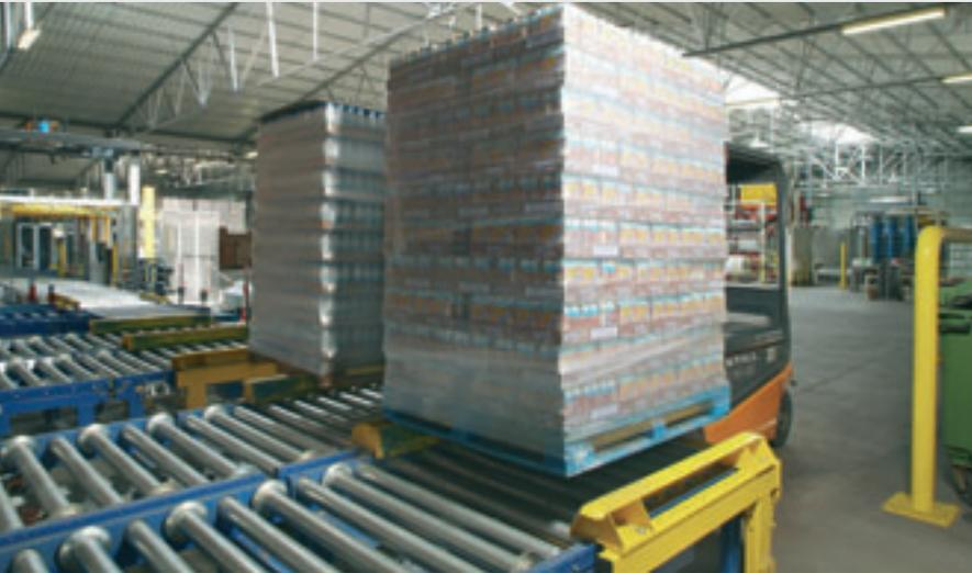
Forklift with double pallet forks puts two pallets onto the conveyor simultaneously
