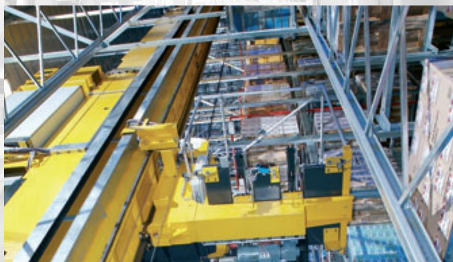
Eleven storage and retrieval machines with telescopic forks for double-deep storage "work" in the high bay warehouse
