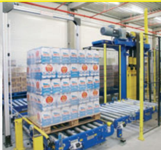
At three i-points, the pallet contour, weight, and data of the transport units are synchronized with the system data.
