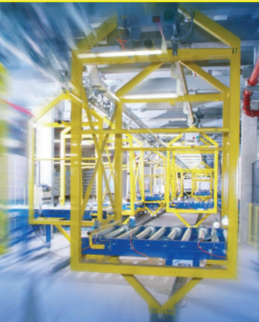
Electric overhead conveyors take the pallets to the shipping area on an oval circuit
