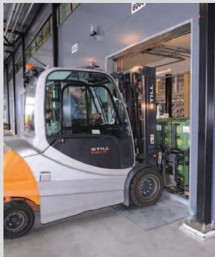
Fork lifts with 3 load handling devices that can load 3 pallets simultaneously are used for loading.
