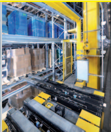
SRM with four telescopic forks for simultaneous acceptance of 2 Euro or one big-box pallet
