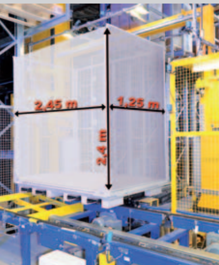
SRM with four telescopic forks for simultaneous acceptance of 2 Euro or one big-box pallet
