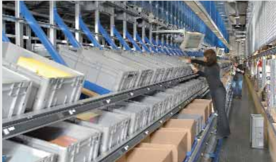
At the pick-positions in the Miniload, goods from totes or from pallets are picked directly into boxes or totes for shipping.
