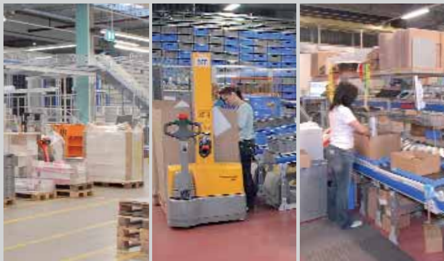
Goods issuing department, order picking onto pallet, into large boxes or packing of smaller packages directly into shipping boxes.
