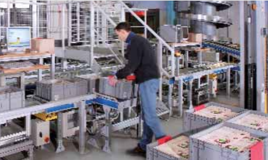
Prior to storing, the goods received for the Miniload (AKL) are repacked in totes.
