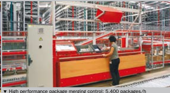
▼ High performance package merging control: 5,400 packages/h
