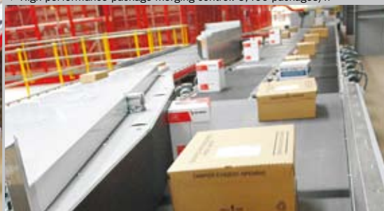
▼ High performance package merging control: 5,400 packages/h
