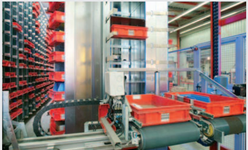
Storage tub retrieval and vertical transport by stationary lifting systems. By eliminating the conventional automatic storage and retrieval systems, the distance between the individual carousels can be reduced and a lot of space saved.
