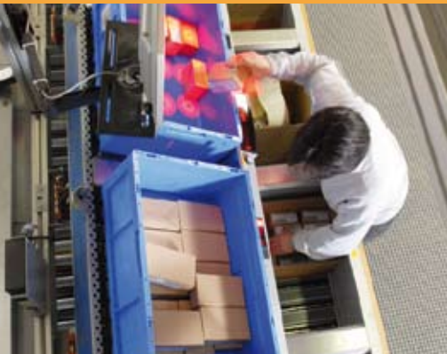
With up to 1,000 to- and from-bin transfers per hour the bins are prepared for picking at two pick-to-tote workstations.
